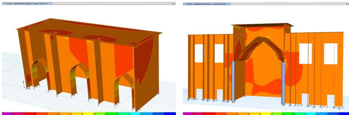
**Figure 14.** The Resulting Bending Moments in the Structural Elements of the Iwans from the ETABS software.
