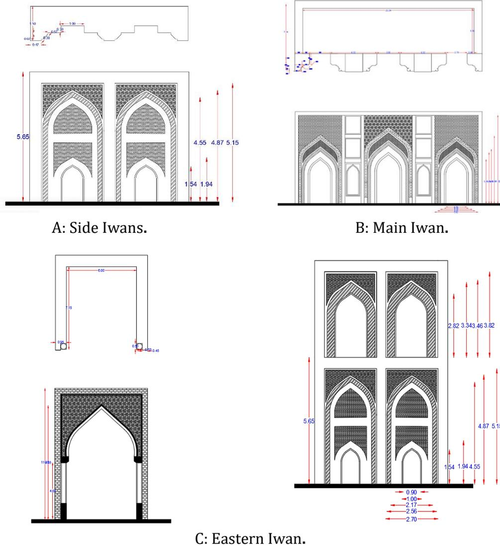
**Figure 8.** The arches that were measured and Redrawn as a Reality.
