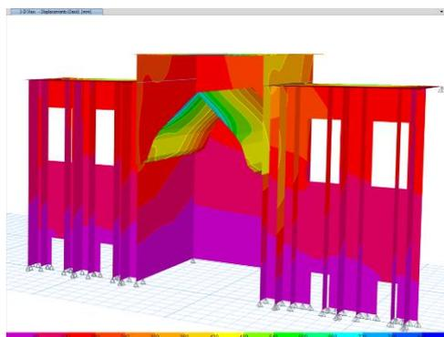
**Figure 11.** The Structural Deviations Resulting from the Structural Elements of the Iwans from the ETABS Program after Raising the Column in the Façade of the Eastern Iwan.
