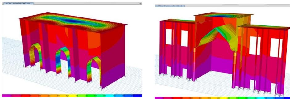
**Figure 10.** Structural Deviations Resulting from the Structural Elements of the Iwans, based on ETABS software.
