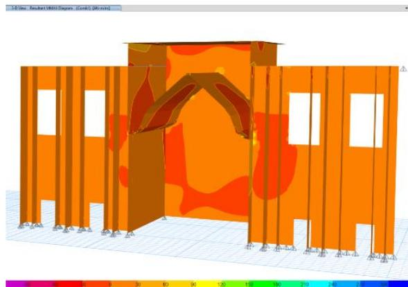
**Figure 15.** Bending Moments Resulting from the Structural Elements of the Iwans from the ETABS Program after Raising the Column in the Facade of Eastern Iwan.
