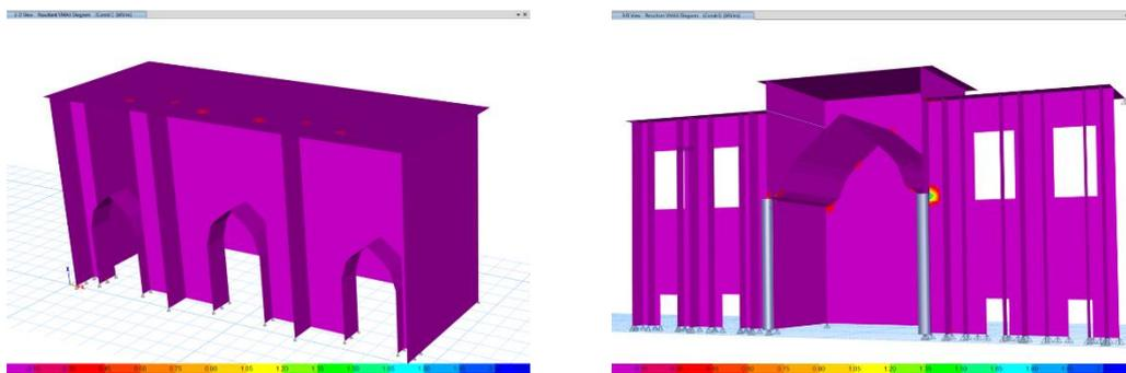
**Figure 13.** Shear Stresses Resulting in the Structural Elements of the Iwans, based on the ETABS software.
