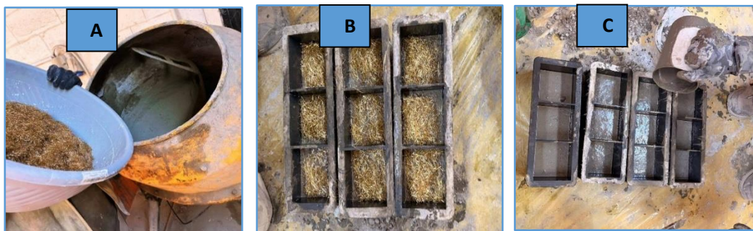
Figure 6. Hybrid mixing technique (A) mix 50 % of fiber directly with dry material (B) 50% of divided into three layers (c) pour the slurry into the mold
