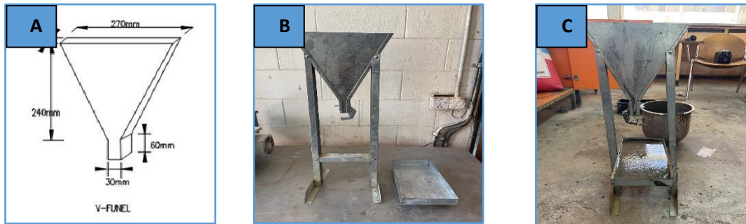
Figure 2. Steps for V-Funnel test for SIFCONs slurry (A) apparatus dimension (EFNARC, 2002), (B) V-funnel (C) measure time in (sec).
