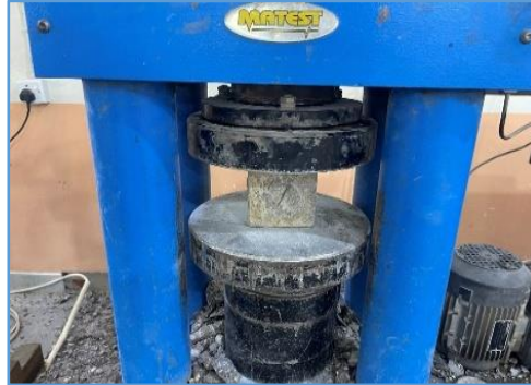
Figure 8. Compressive strength test
