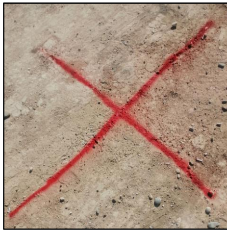
Figure 3. Ground control points (GCPs).
