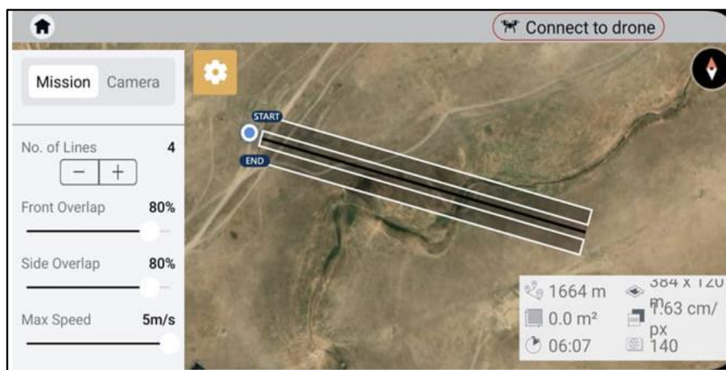
Figure 5. The UAV flight plan showing flight settings.
