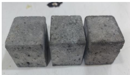
Figure 2. Specimens of mortar
