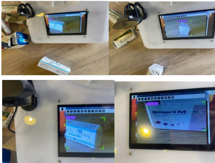
Figure 7. Detection performance for varying viewing angles and visibility of part of the object.
