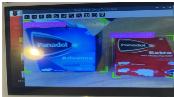
Figure 6. Multi-object medication detection with multiple drugs detected at once with the YOLO model.
