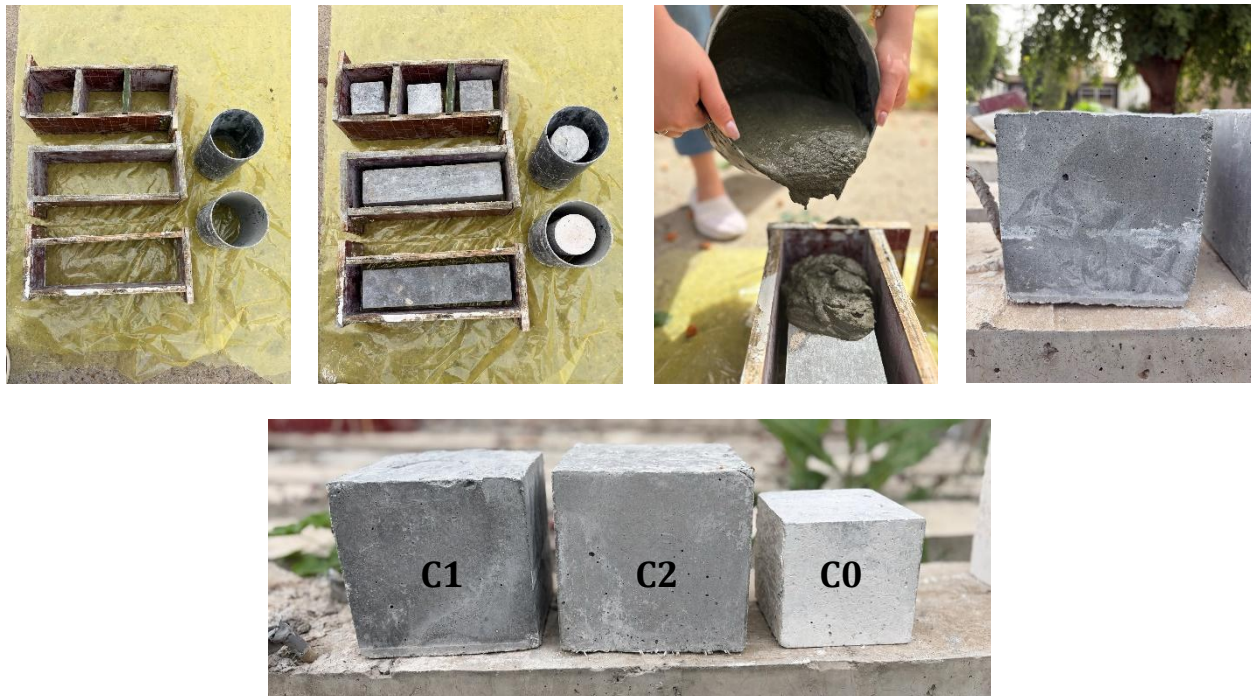
Figure 2. Molding and casting the fire protective coatings
