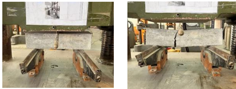
Figure 5. Flexural strength test set up
