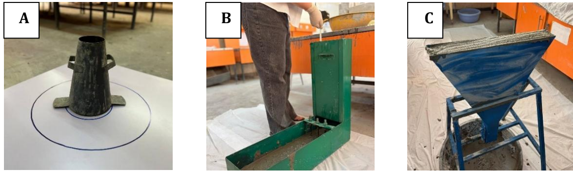
Figure 3. (A) Slump flow test, (B) L-Box test and (C) V-Funnel test
