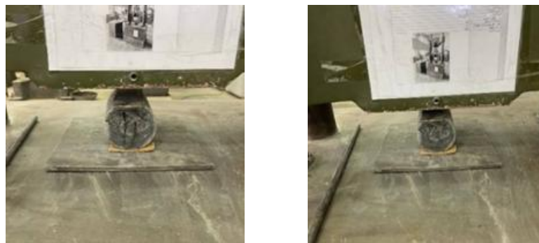
Figure 6. Splitting tensile strength test set up
