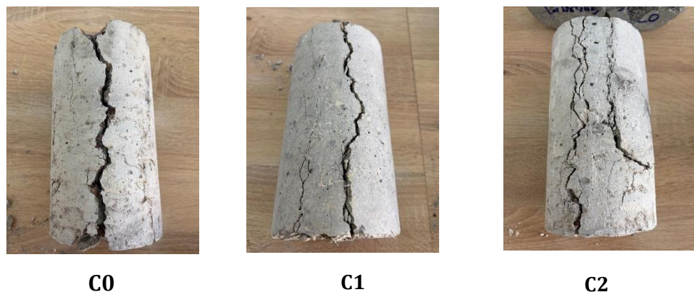
Figure 13. Specimens after fire exposure and splitting tensile strength test
