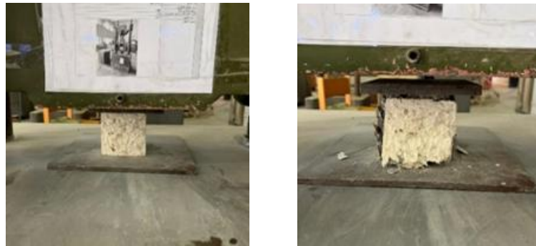
Figure 4. Compressive strength test set up
