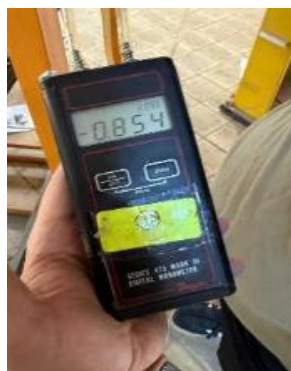
Figure 3. Reference-flow verification and control system: (a) Dwyer Series 475 Mark III digital differential manometer; (b) Pitot-static tube arrangement
