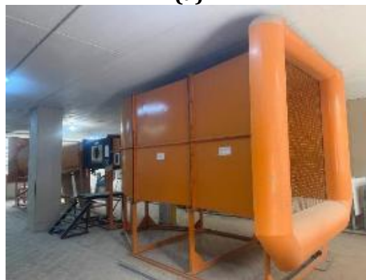
Figure 2. Open-circuit wind tunnel used in the experimental investigation: (a) schematic layout of the tunnel components and roof-model position inside the test section; (b) actual wind tunnel facility at the Department of Aerospace Engineering, University of Baghdad.
