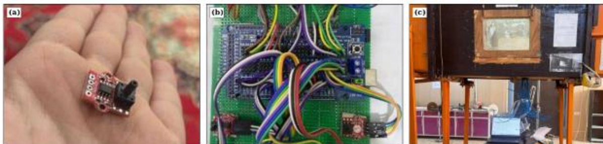
Figure 10. Pressure measurement and data acquisition system: (a) differential pressure sensors; (b) custom-developed acquisition unit; (c) computer-based recording and post-processing arrangement.
