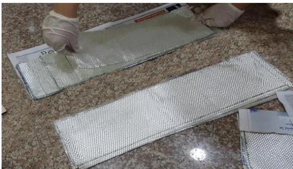
**Figure 5.** Woven glass fiber layers.
