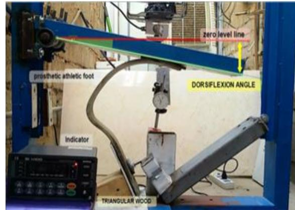
Figure 8. Measuring dorsiflexion angle for design B foot sample.
