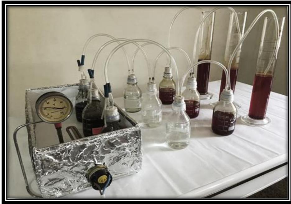
Figure. 1 Digesters arrangement and set up.
