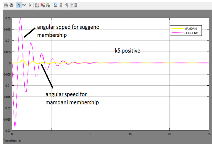
Figure 22. Angular speed for mamdani and sugeno membership function comparison.
