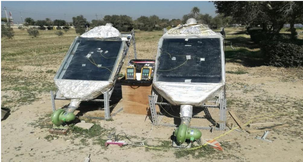
**Figure 8.** Photographic view of sheet of transparent honeycomb (V) (right) and conventional (I) (left) SAH.
