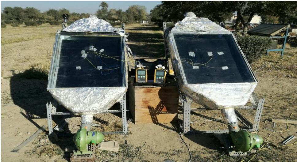
**Figure 5.** Photographic view of dual channel (II) (right) and conventional (I) (left) SAH.
