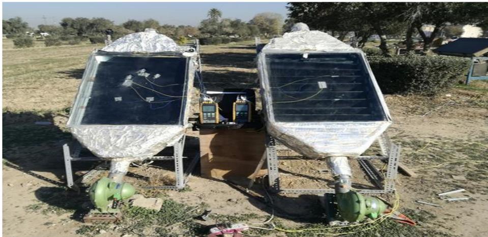
**Figure 6.** Photographic view of perforating “V” corrugated plate (III) (right) and conventional(I) (left) SAH.
