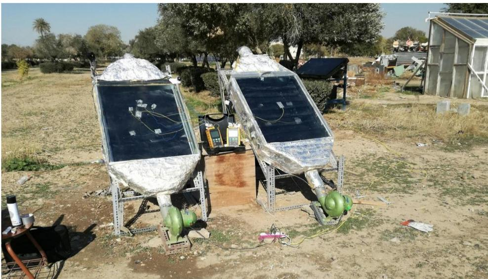
**Figure 7.** Photographic view of wire mesh (IV) (right) and conventional (I) (left) SAH.
