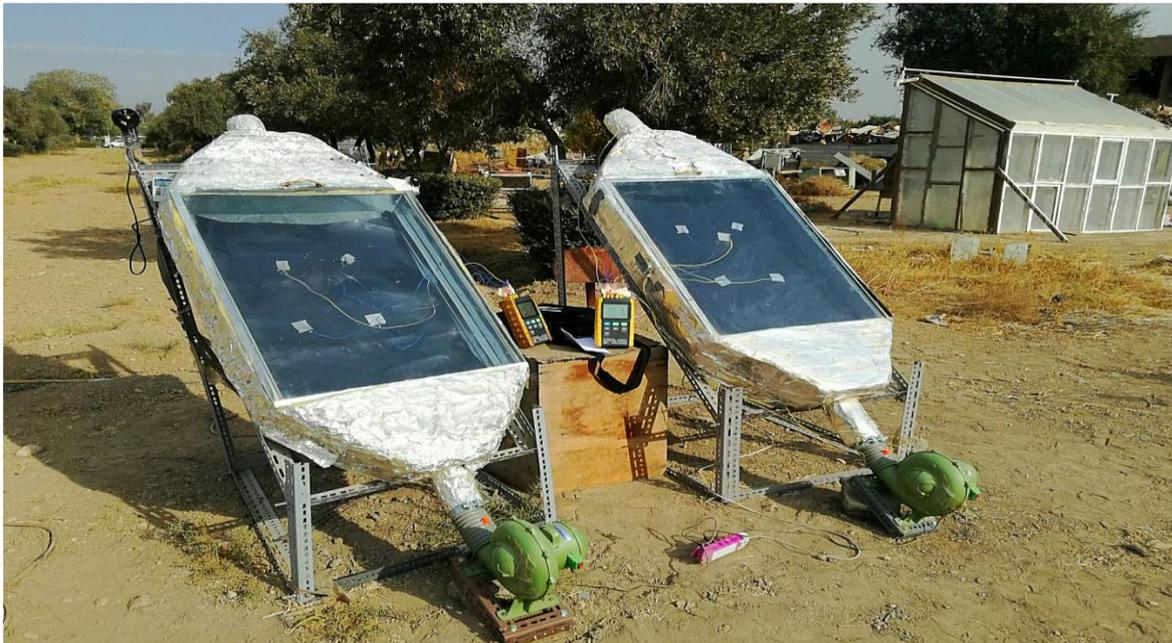
**Figure 1.** Photographic view of experimental setup solar collector.
