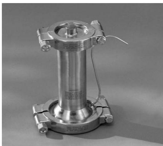
Figure 1. Photograph of the dead-end filtration cell (STERLITECH HP4750).
