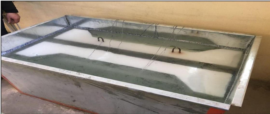
**Plate 4.** Curing of Specimens in Tap Water.
