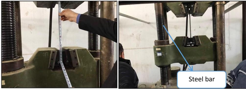
**Plate 2.** Tensile Machine for Steel Bars Testing
