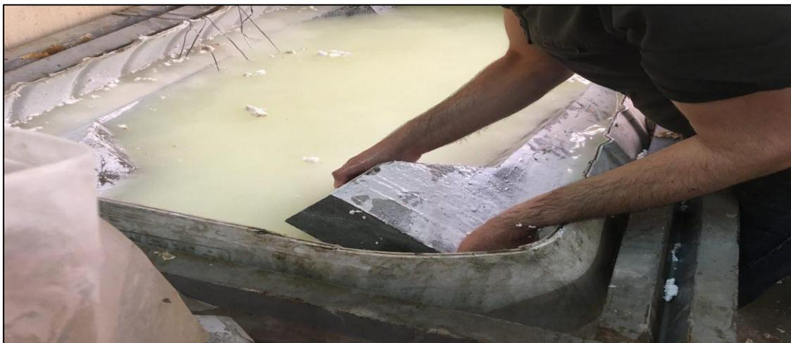
**Plate 5.** Curing of Specimens in Chloride Water.
