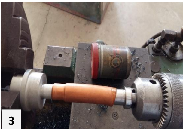
Figure 8. Steps for expanding pipe.
