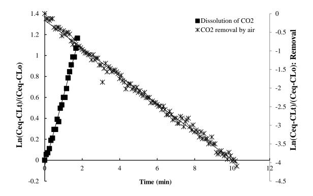
Figure 7. Volumetric mass transfer coefficient in dissolution and removal process with distilled water.
