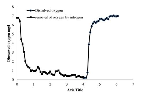
Figure 4. Dissolution and removal of oxygen in the distilled water.
