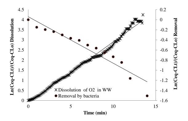
Figure 9. The volumetric mass transfer coefficient of dissolution in wastewater and removal process by metabolic processes.
