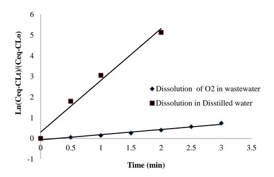
Figure 8. The volumetric mass transfer coefficient of dissolution of oxygen in wastewater and distilled water.
