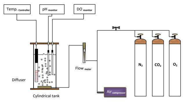
Figure 1. Schematic diagram of cylindrical tank used in mass transfer study.
