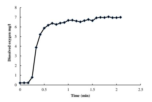
**Figure 3**. The oxygen concentration in distilled water at 30°C when the air was used as gas is sparged.
