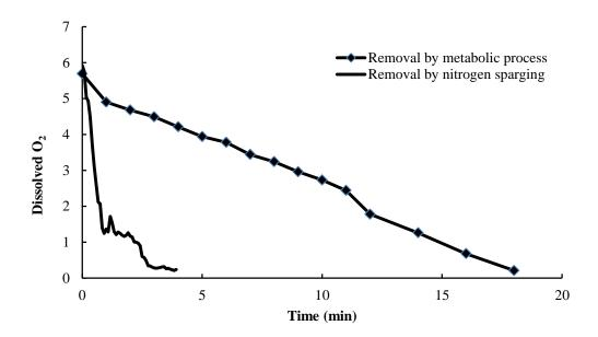
**Figure 6**. Dissolved oxygen in the distilled water, when the bioreactor removed by pure nitrogen, as well as in wastewater when the removal carried out by a metabolic process.
