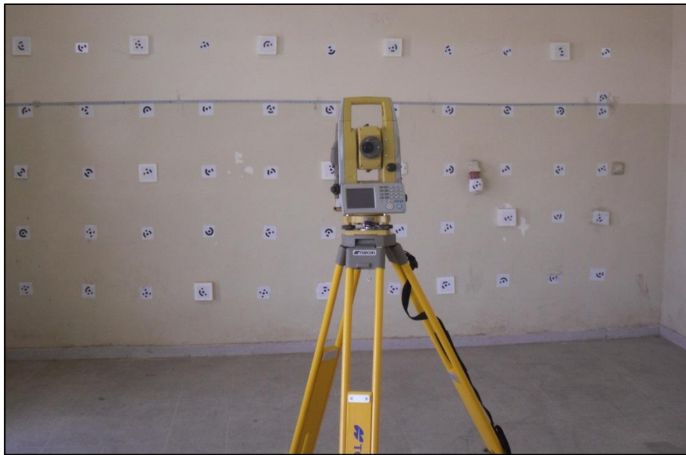
Figure 1. Establishing test field targets.
