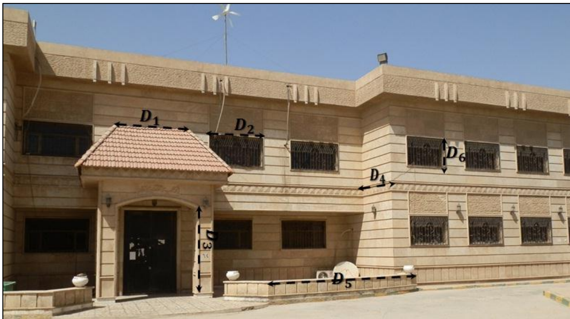
Figure 10. The photos and the 3D view of the six check distances at the outdoor environment.
