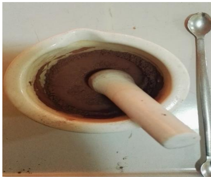
Figure 2. Blending process (Pestle and mortar).
