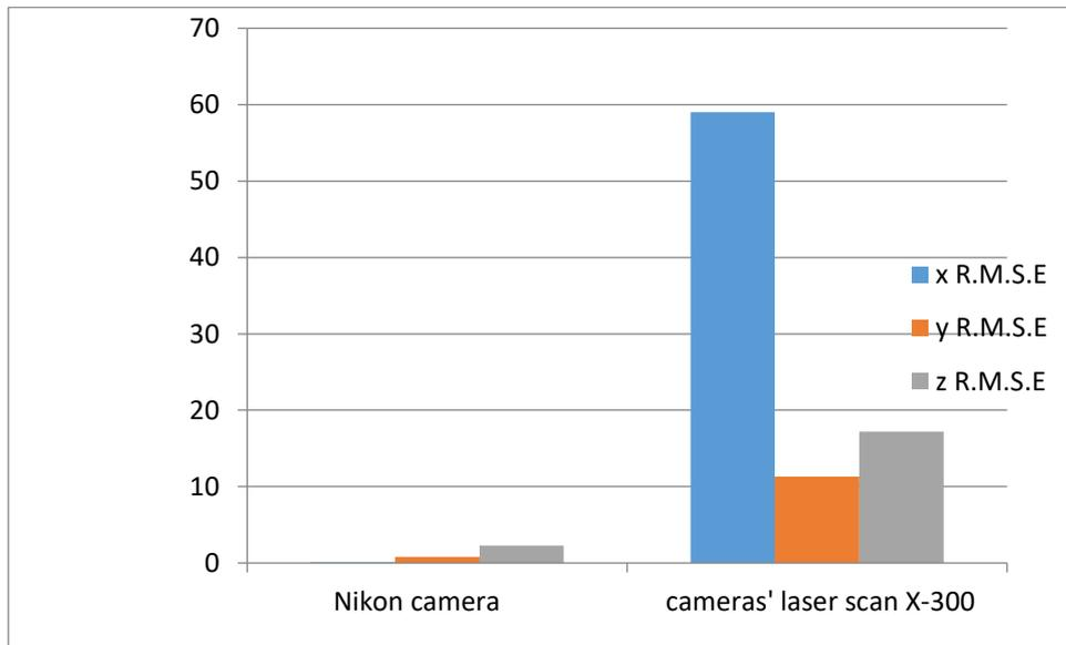
Figure 11. (RMSE) using photos of Nikon camera and photos of cameras' laser scan X-300 by (LPS) software.
