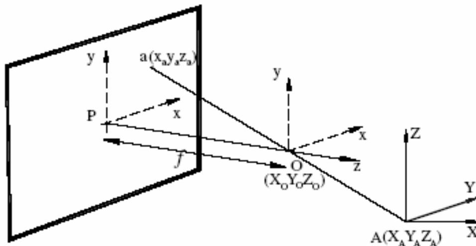
**Figure 1.** Central perspective of point A in close range photogrammetry, Arias, et al., 2005.
