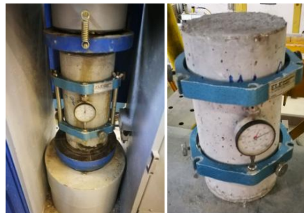
Figure 10. Modulus of elasticity test.
