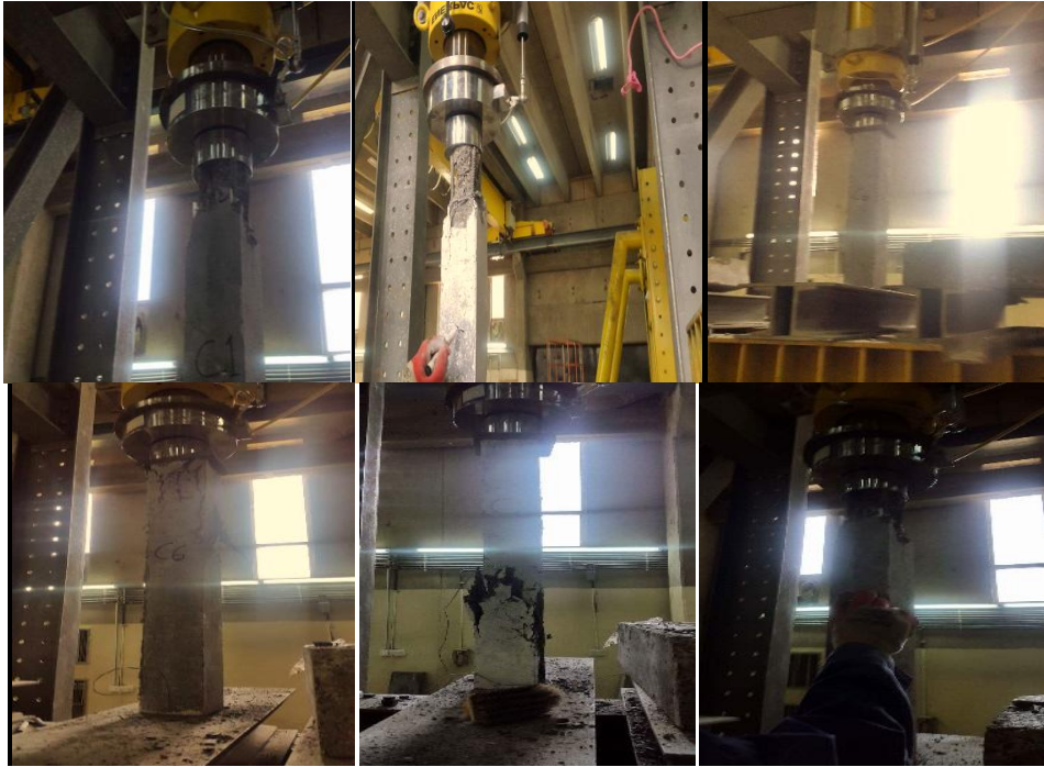
Figure 9. Crack pattern and mode of failure columns.
