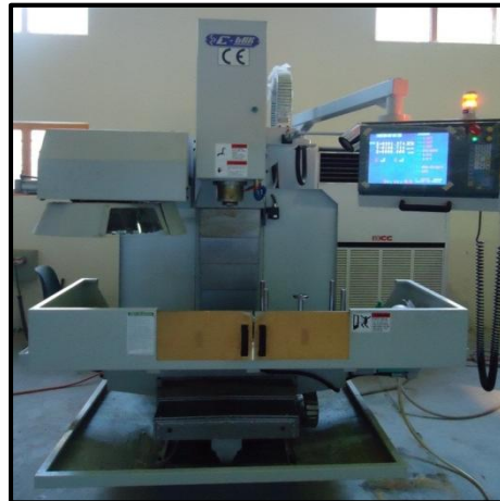
Figure 6. CNC C-TEK 3-axes Milling Machine.
