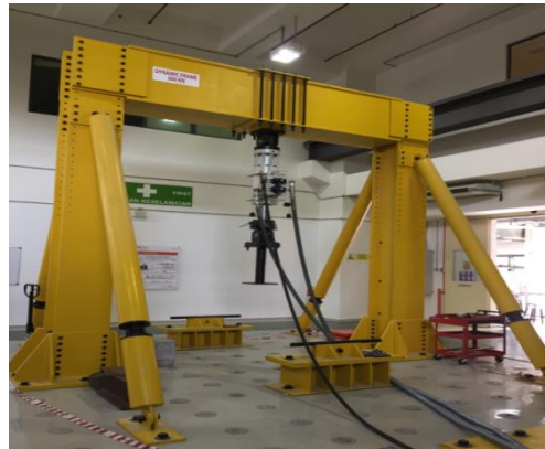
Plate 1. The hydraulic actuators used to test the LRC beams.
