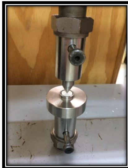
Figure 2. The biaxial flexural strength test
