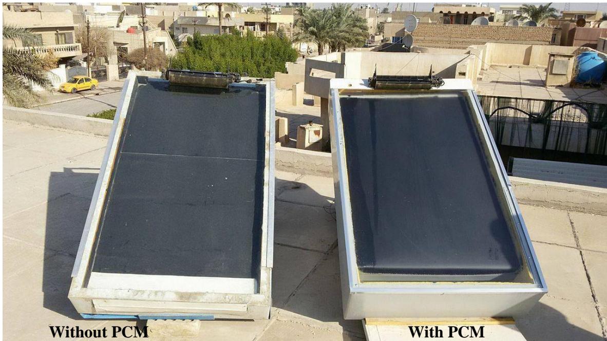
Figure 2. A photographic image of the double pass solar air heaters (with and without using PCM).
