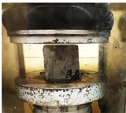
(a) Testing concrete cubes
