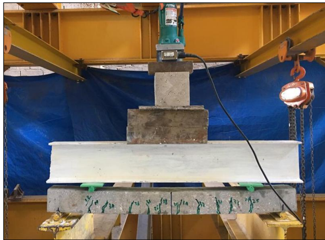
Figure 8. Cracks Propagation in control beam specimen.
