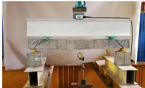
Figure 11. Cracks propagation and failure mode of beams with full adhesion at segments interface.
