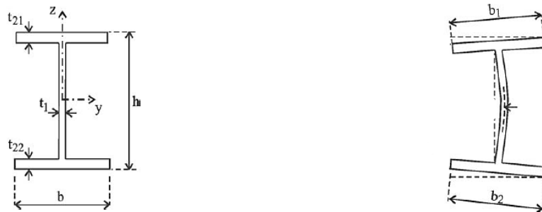
a- Geometric characteristics h, b, t_1, t_{21}, t_{22} . b- Geometric characteristics b_1, b_2 .
