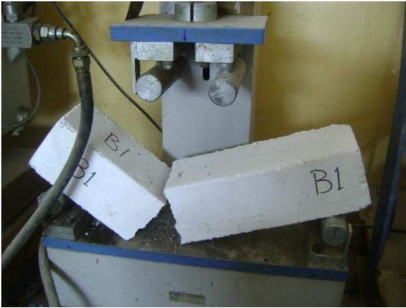
Figure 7. Failure of original beam B1.
