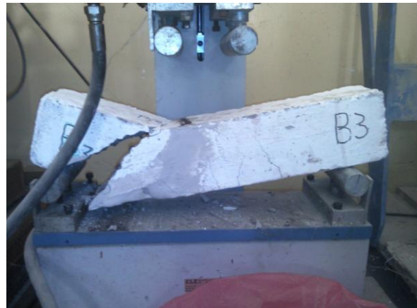
Figure 12. Failure of B3 after repair.
