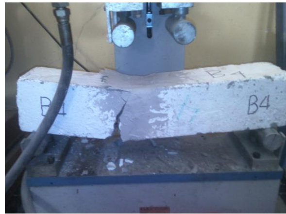
Figure 14. Failure of B4 after repair.
