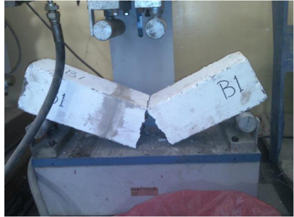
Figure 8. Failure of beam B1 after repair.
