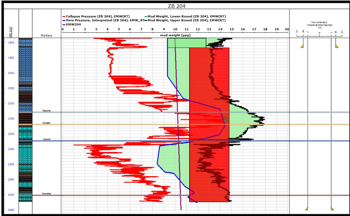
Figure 7-a. Previous mud weight and casing programs.
