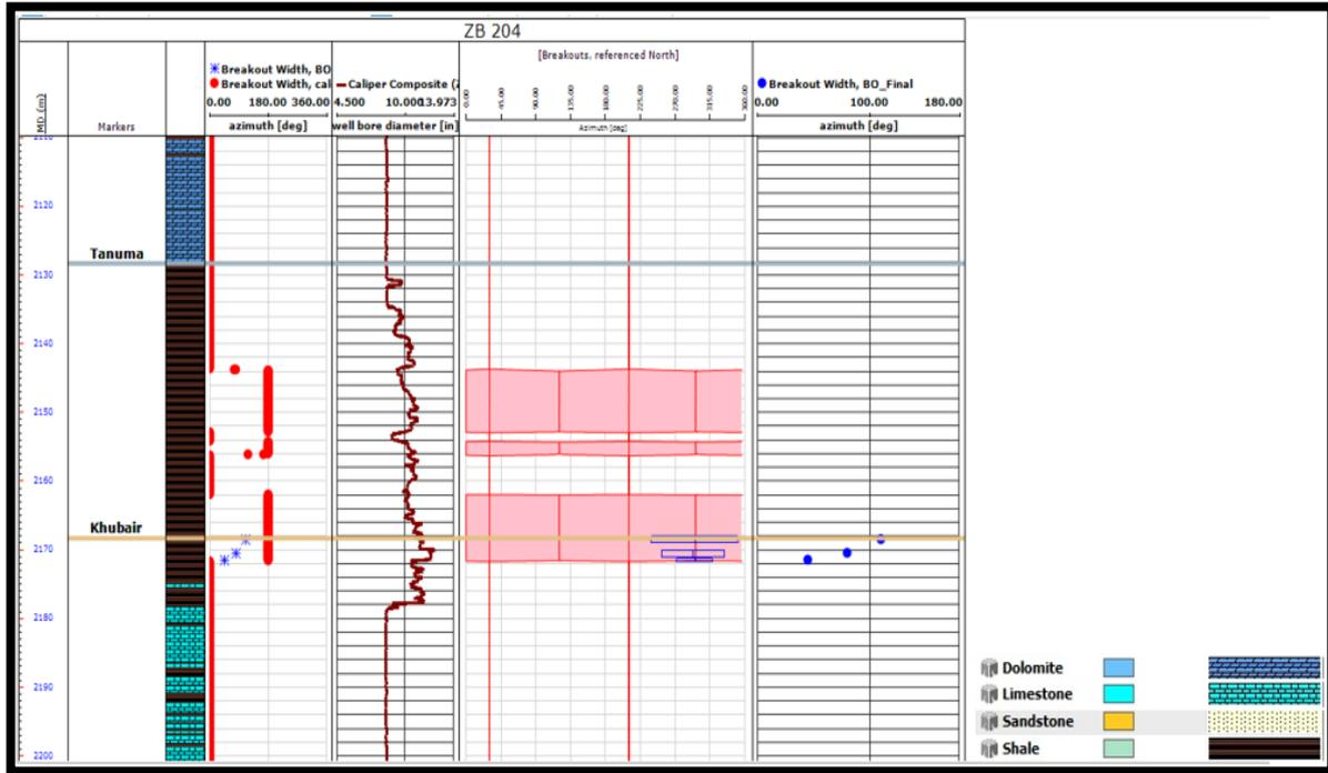
Figure 3. Breakout azimuth profile.
