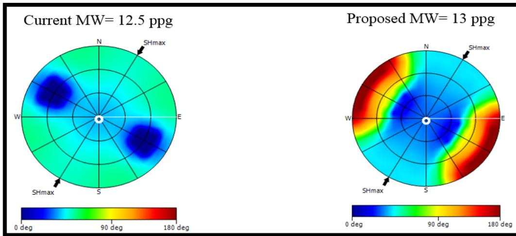
**Figure 6-c.** Effect of direction of drilling on the breakout width, Mogi-Coulomb failure criteria.
