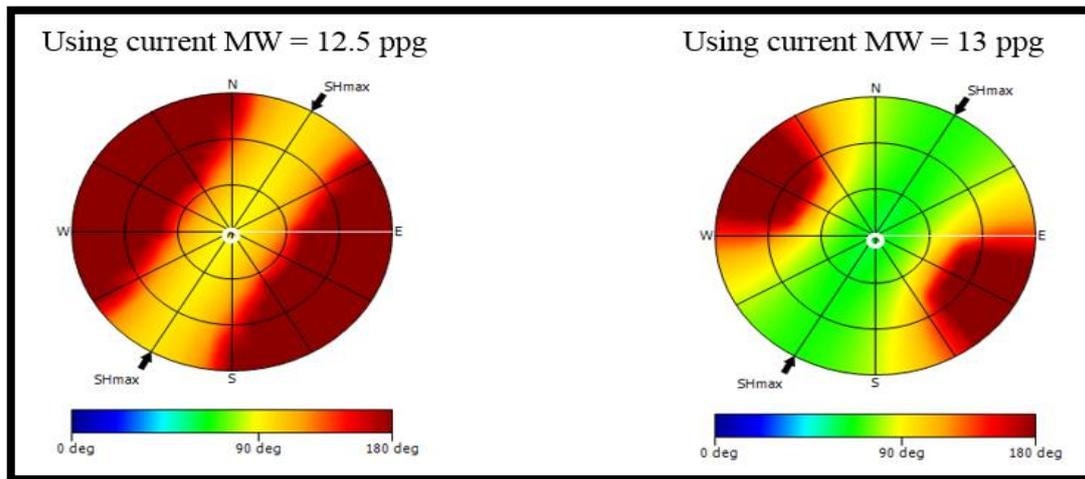
Figure 6-a. Effect of direction of drilling on the breakout width, Mohr-Coulomb failure criteria.
