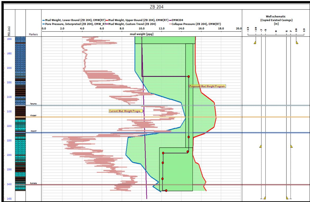
Figure 7-b. Suggested mud weight and casing programs.
