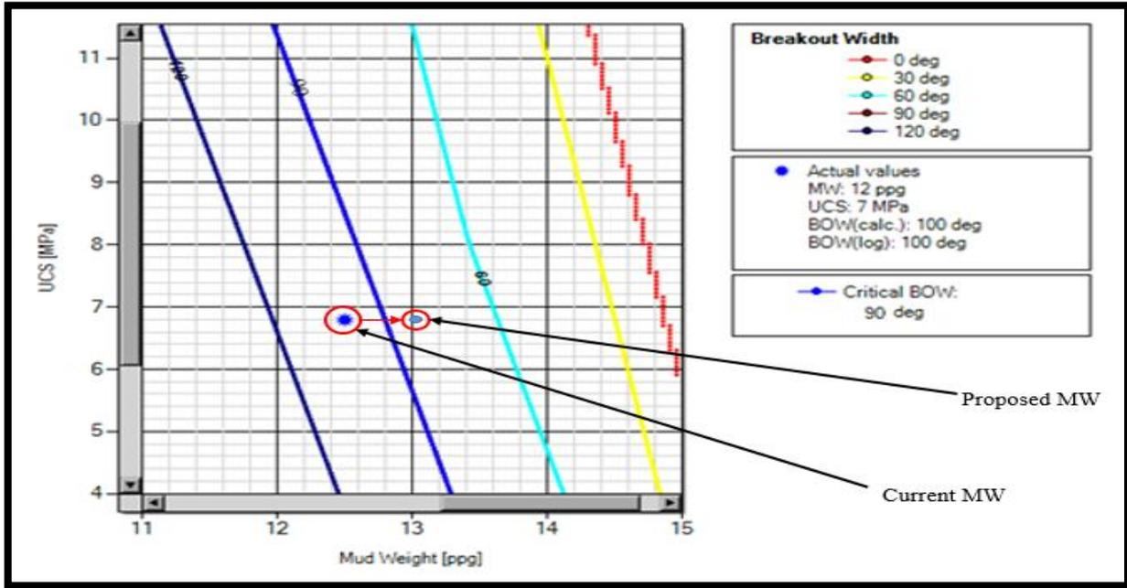
Figure 5. Breakouts as a function of Mud Weight and UCS.
