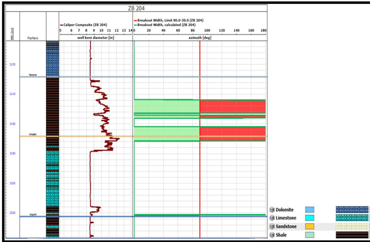
**Figure 2.** Predicted breakout width profile.
