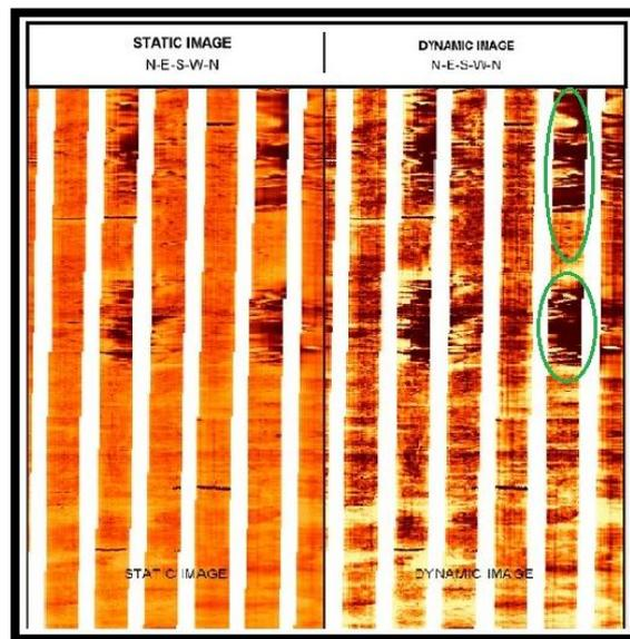
**Figure 1.** XRMI image log shows obvious breakouts, (final well drilling reports, 2011).
