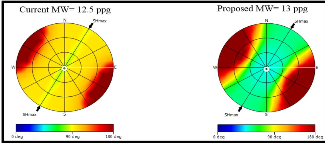
**Figure 6-b.** Effect of direction of drilling on the breakout width, Modified Lade failure criteria.
