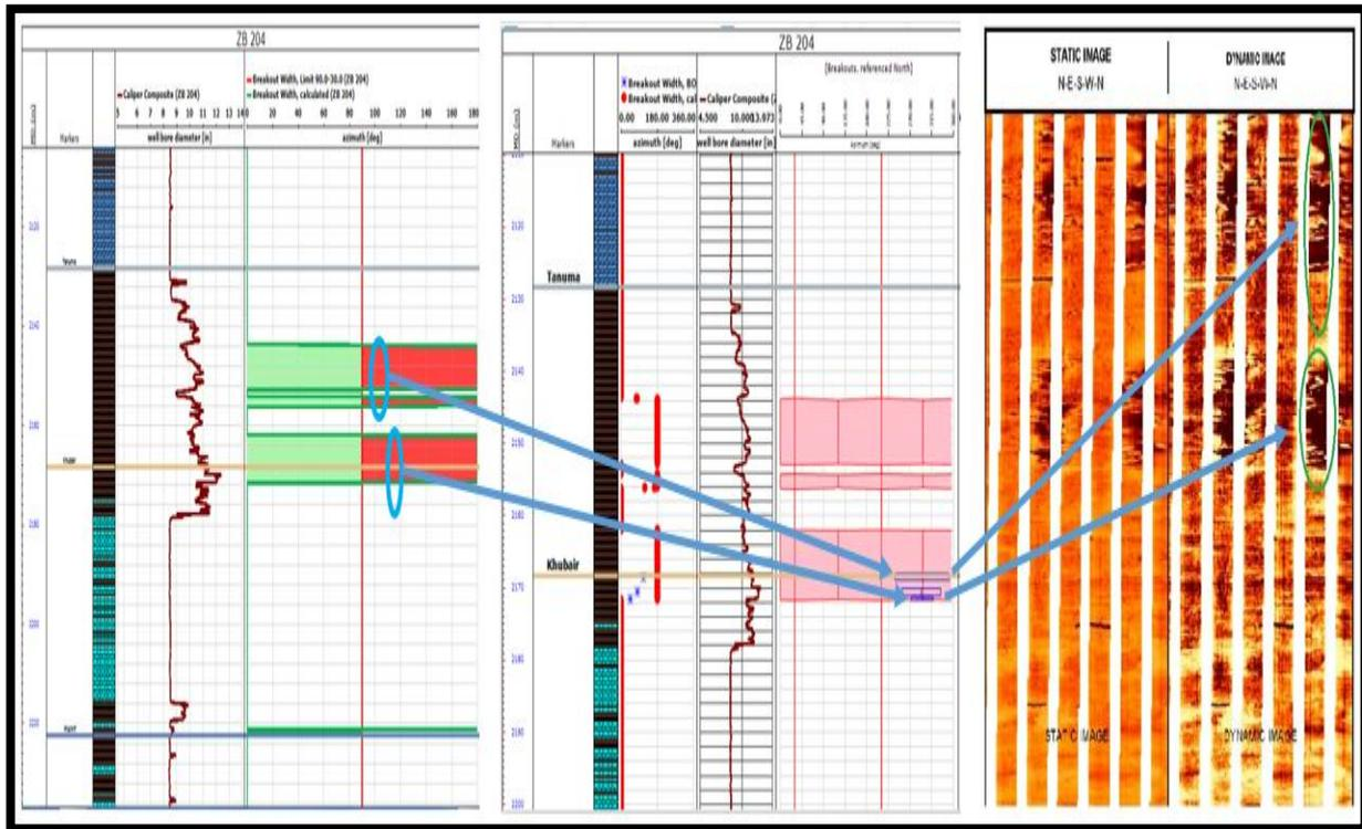
Figure 4. Breakout prediction and calibration (Figures 1,2 and 3 gathered).
