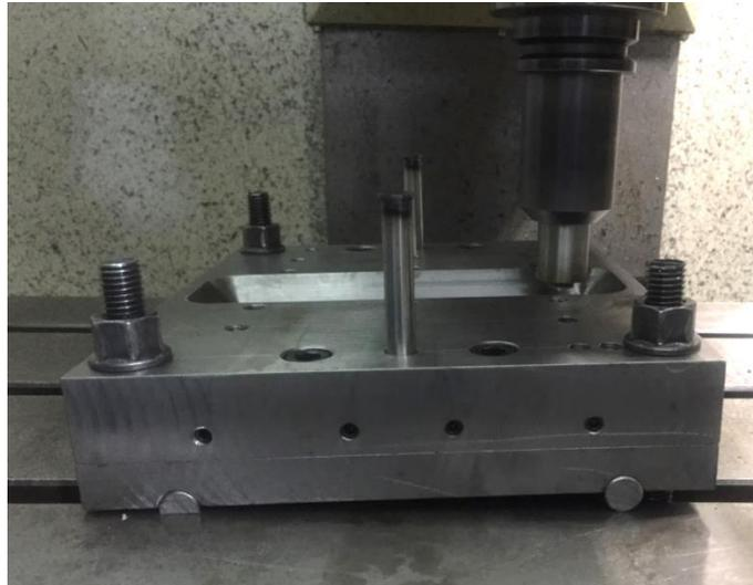
**Figure 2.** The backing plate and fixture tilted in  $2^\circ$  set up on the table of the machine.
