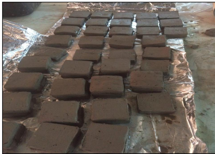
Plate 2. Reconstituted soil specimens prepared for Thixotropic effects investigation.
