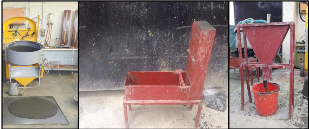
Figure 3. Fresh properties tests: (a) slump flow, (b) L-box, (c) V-funnel.
