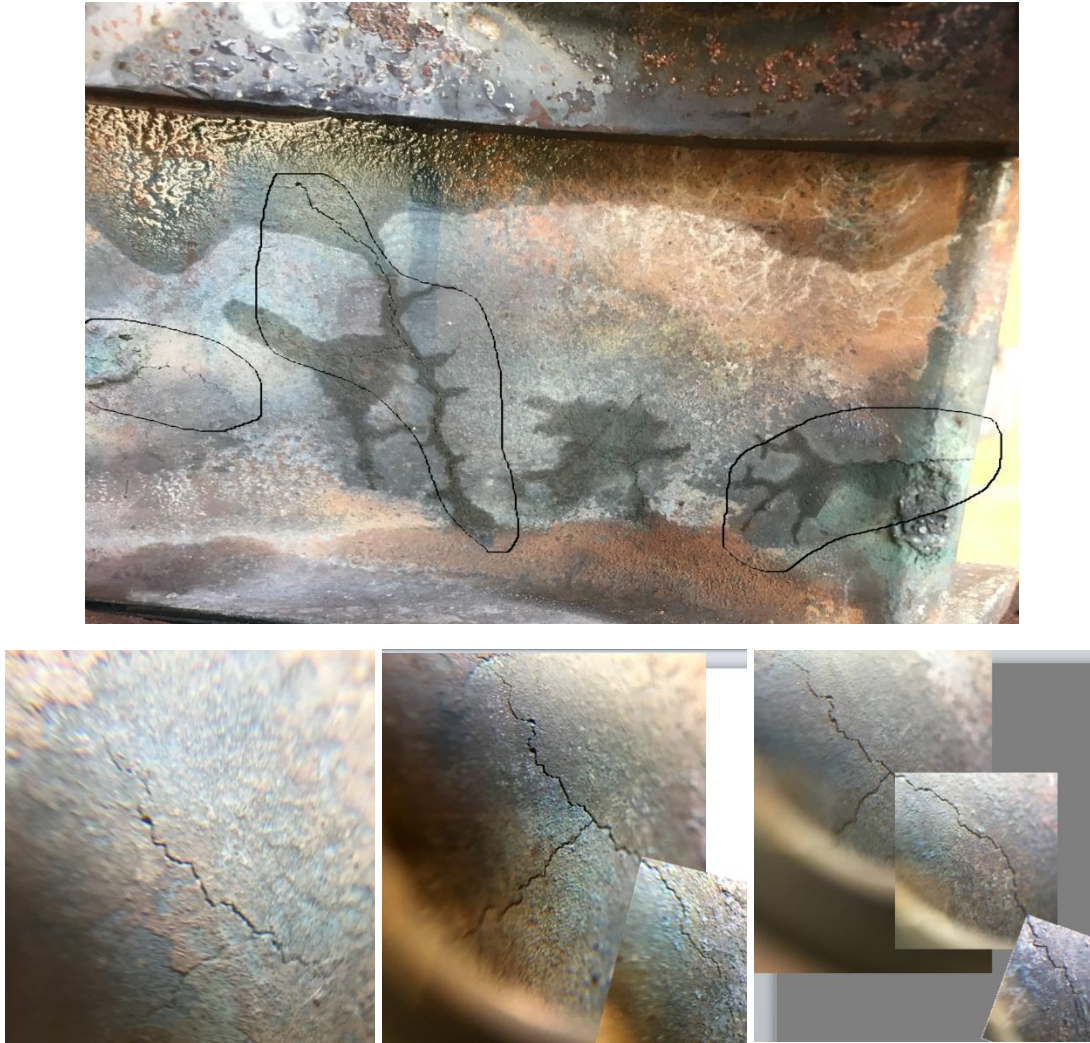
Figure 25. The failure blade after 460 cycles.
