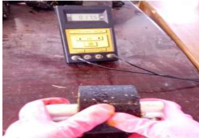
Plate 2. Ultrasonic pulse velocity test setup.
