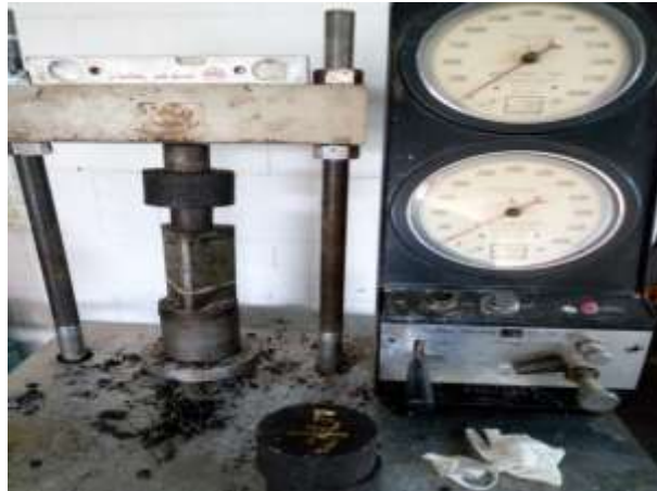
Plate 3. Tensile strength test setup.
