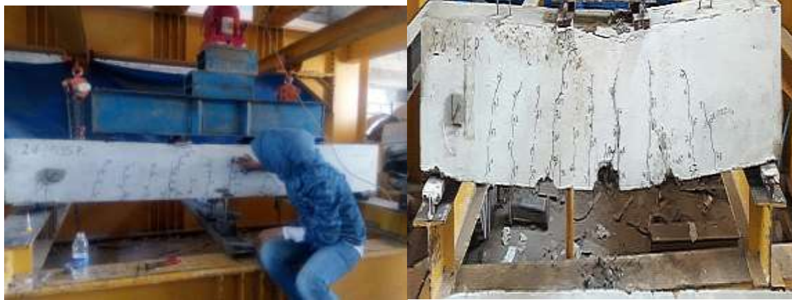
Figure 3. The first RC beam testing.
