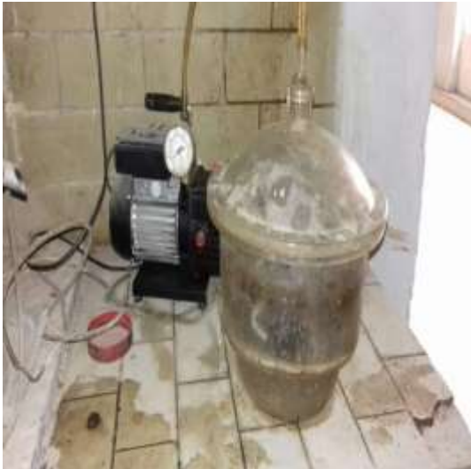
a-Vacuum process for specimens
